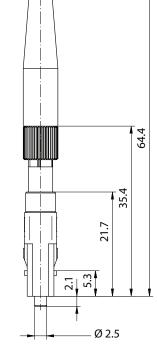
Pic. 2 Dimensions SC clamp connector without grip plate
