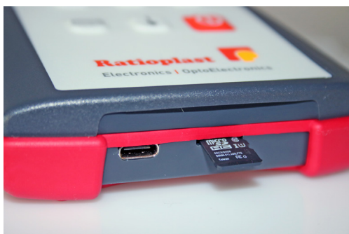
Pic. 8 USB interface and microSD card slot
