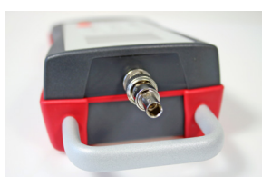
Pic. 3 BNC socket with F-ST adapter 909MS660ST001
